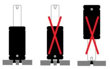
Mount the gas spring on perfect flat surface. Ensure the bolts are tight and spring cannot move during use. Do not use piston hole taping for mounting the spring, it is only for maintenance purpose
