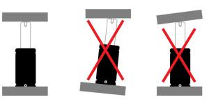
Mount the gas spring between two perfectly parallel surface to ensure maximum life. Mounting gas spring in non parallel surfaces could lead to significant decrease in life.
